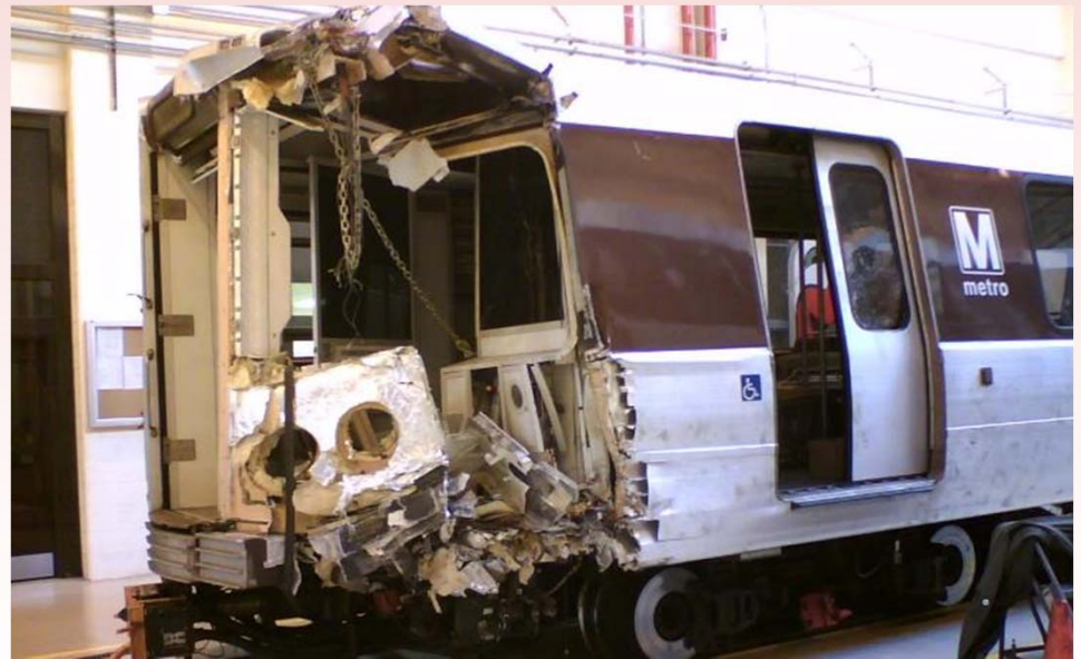
2007 Metro derailment due to wheel climb, photo by by Keon T., Wikipedia (CC BY-SA 2.5) Literature: National Transportation Safety Board Derailment of Washington Metropolitan Area Transit Authority Train near the Mt. Vernon Square Station Washington, D.C. January 7, 2007, https://www.nts.gov/doclib/reports/2007/RAR0703.pdf
